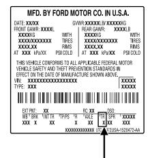
You can find a transmission/transaxle code on the vehicle Safety Compliance Certification Label. The following table tells you which transmission or transaxle each code represents.
